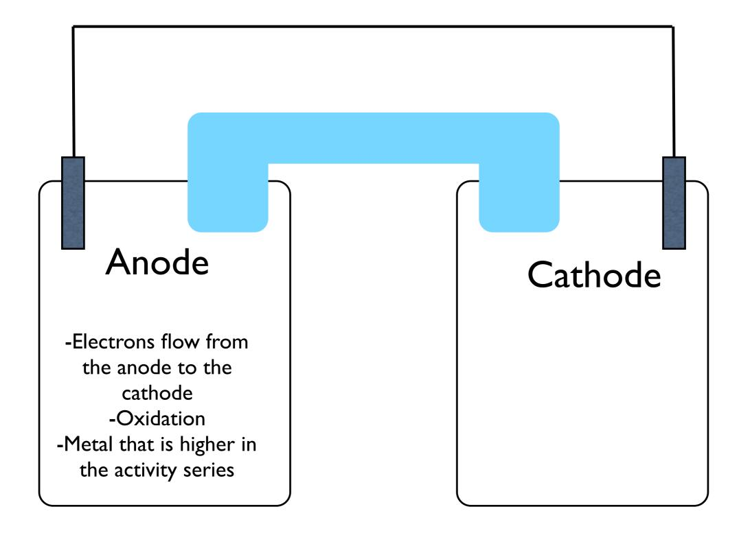
Create a diagram of a Galvanic cell using copper and nickel
